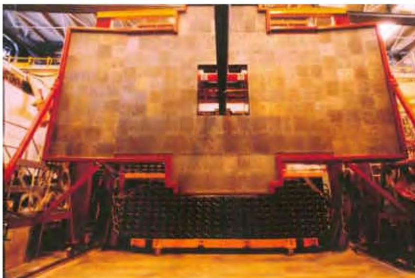
The WA98 PMD at the CERN SPS, viewed from the lead converter side.
