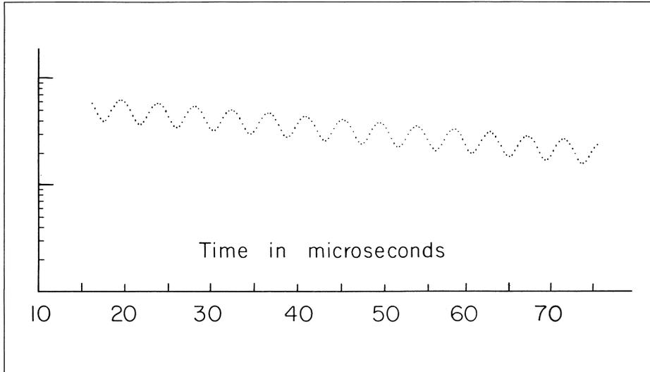
trajectory, which takes about 4 microseconds. It is this modulation period which must be measured very precisely, to 1.3 picosecond.
