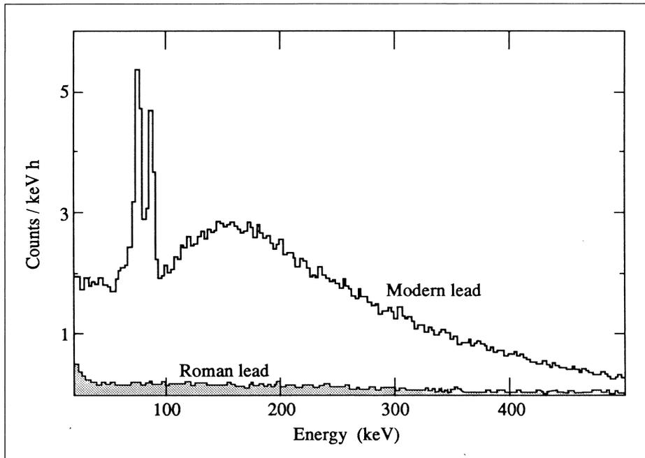
py was also carried out for comparison on samples of modern lead, on specially-produced low radioactivity lead and on a sample of lead about 500 years old.
